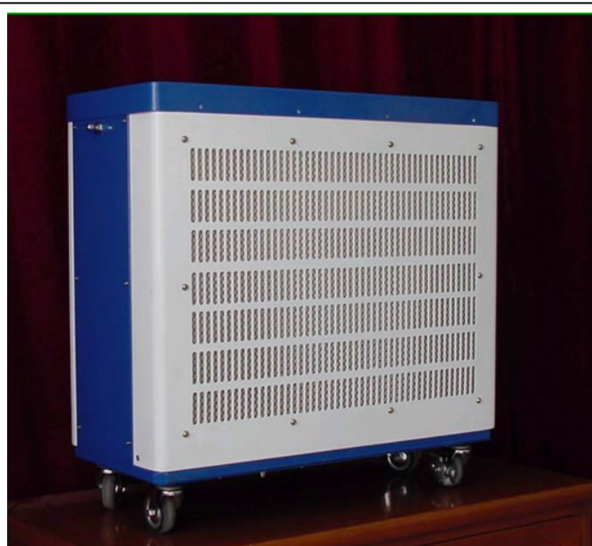
Figure 1. This recent, "light-weight" 2 kW PEMFC system (stacks, compressor, regulators, controller, no storage), at 50 kg, is more massive than a 20-year-old 2 kW diesel gen-set. Its price has increased by 21% to $17,000 during the past year [2].
