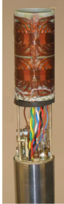
NB MRI Probe with 26-40 Gradients and an RF coil
